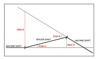
Figure 7. Methods for specifying maximum angle allowed between spacer shaft and connected machine shafts
