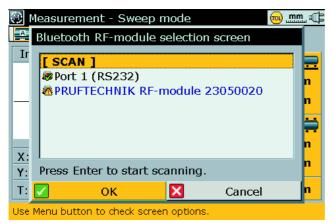
Note: Up to a maximum of 5 RF modules previously detected by the instrument, always appear on the selection screen.
